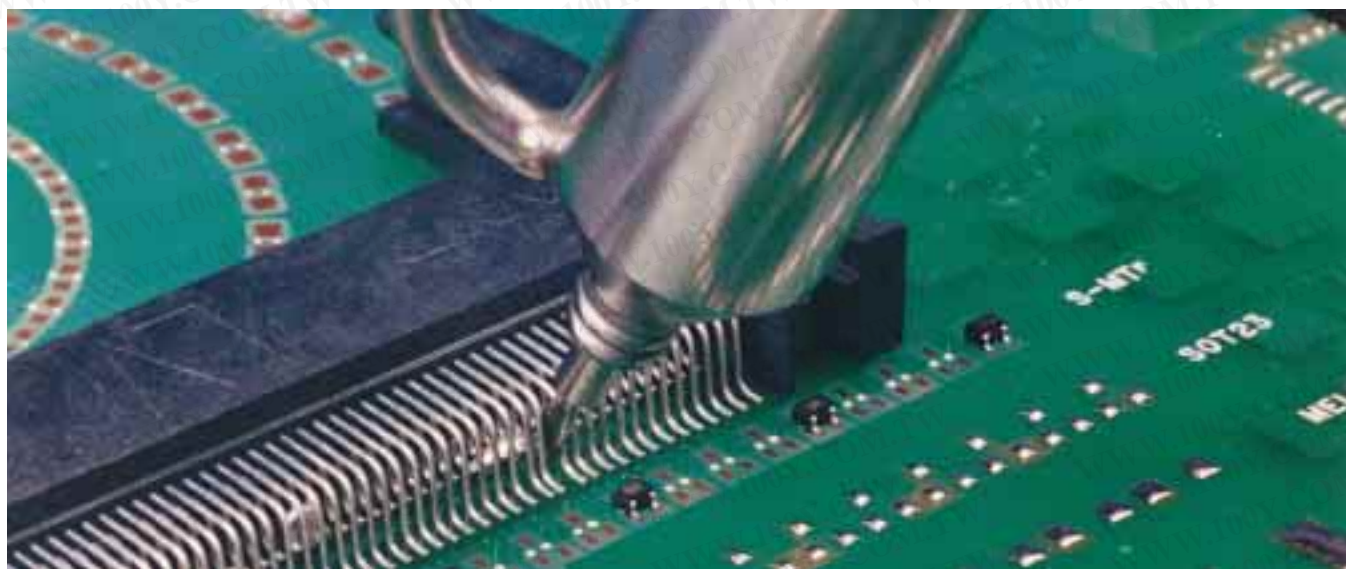
The TSX70, with the TSX717 tip, can be used for reaching components partially hidden or located in crowded areas.
