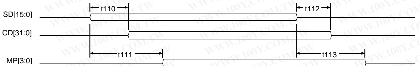
Figure 6-5 SD[15:0] to CD[31:0] and MP[3:0] Valid and Invalid Delay
