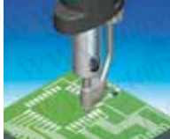
Cleaning pads with desoldering iron
