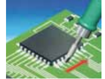
Soldering leads with special JBC series tips for soldering SMDs
