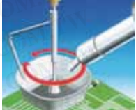
Desoldering IC component with hot air
