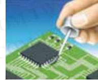
Fluxing IC pads and leads
