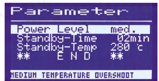
Safe control is possible when temp sensitive components require NO OVERSHOOT! - power level “low”!
