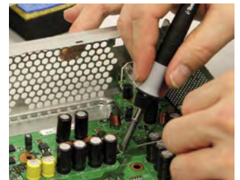
High-mass SMD soldering in hard-to-reach areas
