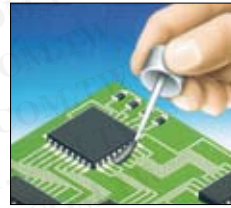
Fluxing the IC pads and leads with flux.
