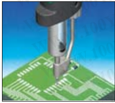
Cleaning the pads with desoldering iron.
