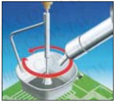
Desoldering the IC component with hot air.
