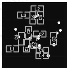
Figure 25. Bottom Layer Silkscreen
