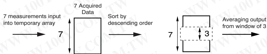
Figure 28. MAV Filter Operation (Patent Pending)
