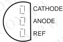
TL431, TL431A, TL431B . . . LP (TO-92/TO-226) PACKAGE (TOP VIEW)
