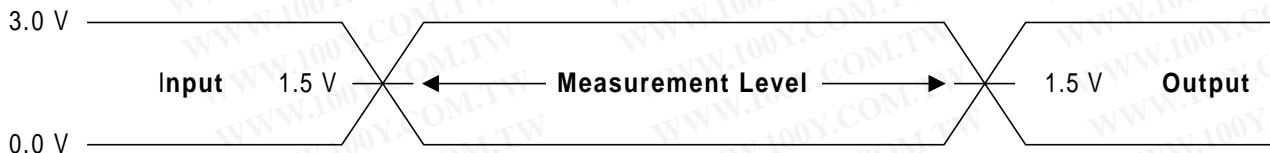
Figure 14. Input Waveforms and Measurement Levels
