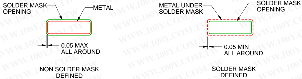
SOLDER MASK DETAILS NOT TO SCALE
