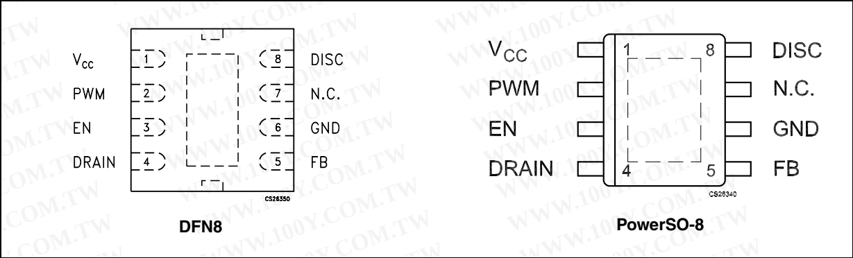
Figure 2. Pin connections (top view)
