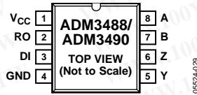
Figure 5. ADM3488/ADM3490 Pin Configuration
