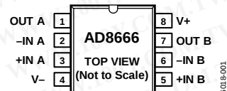
Figure 3. AD8666, 8-Lead SOIC_N (R-8)
