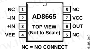
Figure 2. AD8665, 8-Lead SOIC_N (R-8)
