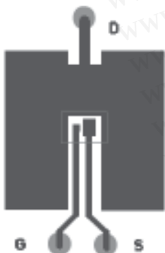
③ Surface mounted on 1 in. square Cu board (still air).
