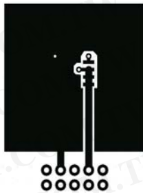
a) 50^\circ\text{C/W} when mounted on a 1\text{in}^2 pad of 2 oz copper.
