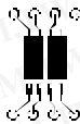
b) 125^\circ\text{C/W} when mounted on a 0.02\text{ in}^2 pad of 2 oz copper
