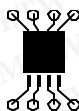
b) 105^\circ\text{C/W} when mounted on a .04\text{ in}^2 pad of 2 oz copper
