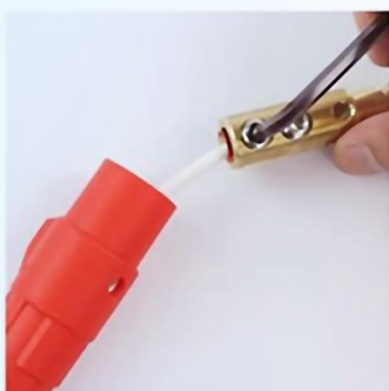
4. 将电线穿入外壳内连接铜片并拧紧螺丝
