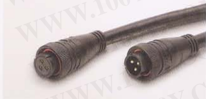
单端预铸电缆-插头 Single-Ended Cordsets--Plug 与SP1711,SP1712,SP1715 相配 Mate with SP1711,SP1712,SP1715
