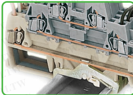
The ground conductor or shield terminal blocks have a ground conductor or shield terminal blocks have a direct contact in the bottom level, automatically establishing direct contact to the carrier rail. The flexible marker carrier, which is placed above the wiring levels, can be pushed aside during wiring or commoning. The marker carrier has three levels for three different WMB markers relating to the three decks of the terminal blocks. With a terminal block width of only 5 mm/0.197 in an effective width of only 1.67 mm/0.066 in for terminal blocks of same or different potentials can be realized for wire sizes 0.08 mm 2 - 2.5 mm 2 (AWG 28 - 14).
